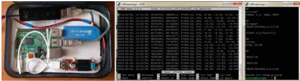
7. Mobilna platforma rejestrująca fale radiowe (Raspberry Pi + DVB-T)[11] Mobile radio wave recording platform (Raspberry Pi + DVB-T)[11]
